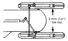
The handlebar should also be horizontal when the skis are pointed toward the front.
