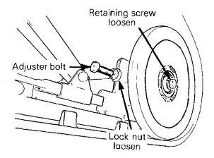
**NOTE:** Track tension and alignment are inter-related. Do not adjust one without the other.
