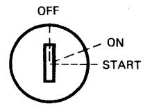
Key operated, 3 position switch. To start engine, turn key fully clockwise to START position and hold. Return key to ON position immediately when engine has started. To stop engine, turn key counter-clockwise to OFF position.
