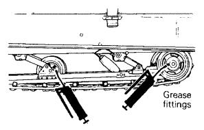
It is recommended that the steering system and suspension be lubricated monthly or every 40 hours of operation. If the vehicle is operated in wet snow or in severe conditions these items should be lubricated more frequently.
