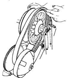
5. Lift the countershaft upward approx. 50 mm (2 in.) and slip the belt between the shaft and the bearing cage to remove completely.
