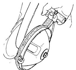
WARNING: Do not wind starting rope around your hand. Hold rope by the handle only.
