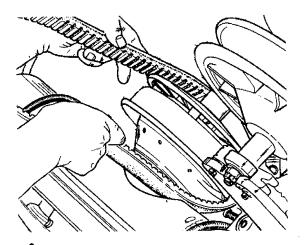
WARNING: After drive belt installation, always check that the brake disc is correctly installed between the brake pads and that the brake is well adjusted. Check brake light operation.
