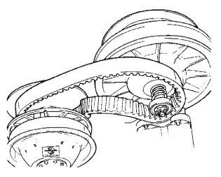
**NOTE:** It may be necessary to loosen the brake adjustment in order to easily lift the countershaft.
