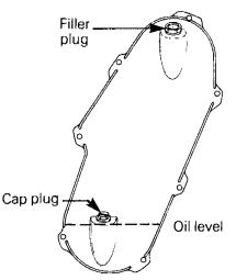
The oil should be level with the bottom of the oil level orifice.
