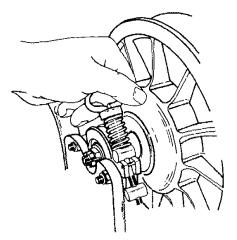
3. Open the driven pulley by twisting and pushing the sliding half. Hold in fully open position.
