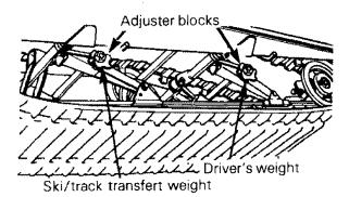
When the front adjuster blocks are at the lowest elevation more weight is distributed on the skis.
